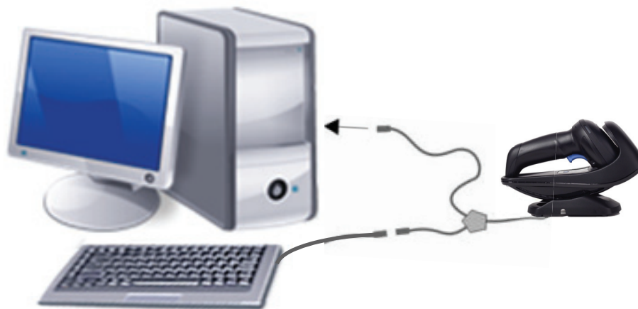
Figure 12 - Connecting to the Host
